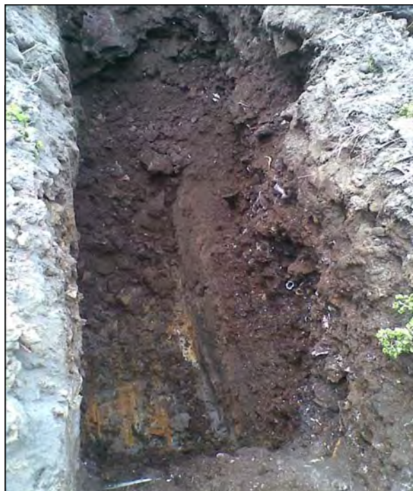
Photograph 4: Test pit TP4 showing metal fragments at about 0.2m to 1.0m
